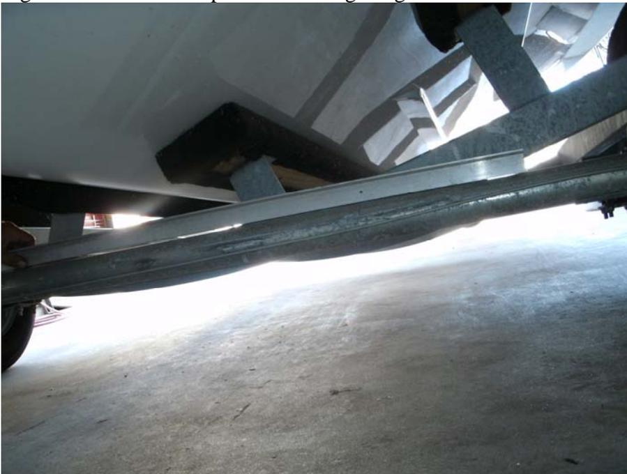
5. Check bearing end play at each tire by jacking them up individually so that they clear the ground. Attempt to rock the wheel back and forth at the 12 and 6 o'clock orientation, and again at 3 and 9 o'clock orientation. If the tire moves more than 1/8", bearings, lug nuts, or other suspension parts are too loose.
